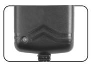
2. When the battery fully charged. The green light will light up and the red light will go out.
